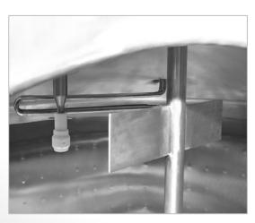
The element requires single phase power. It should be positioned in the tank angled to the center making sure it does not interfere with the agitator shaft or CIP spray balls.
